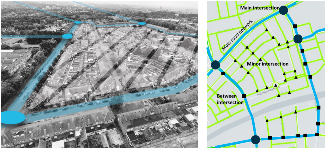
Figure 3: an example of how the VIA Clustered Road Network (VCRN) algorithm fully automated divides the complete nationally road network into clusters of intersections and road sections to combine different data types into a mutually comparable reporting level. Left an aerial photo with the main road network highlighted; right the map with main intersections, between intersections and minor intersections.
